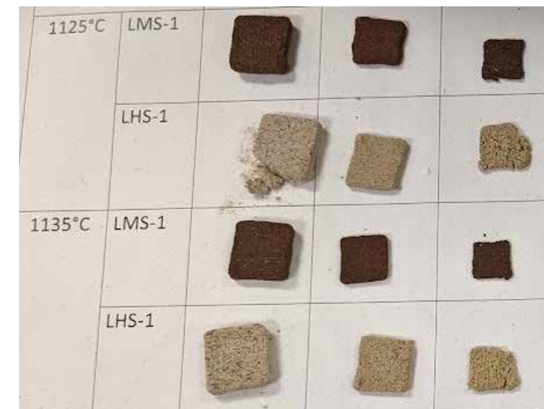
> Some of the high-porosity lunar samples being produced using additive manufacturing. Lunar mare simulants are the darker samples and the lighter samples are constructed from materials representative of highland regions.
